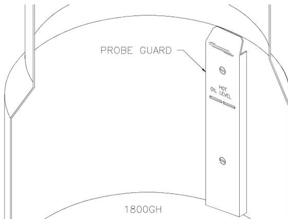
**CAUTION** Using too much force in this area could result in damage to either the hi-limit capillary or the temperature sensor probe. If either of these components are damaged, the unit will be inoperable until the component is replaced.
