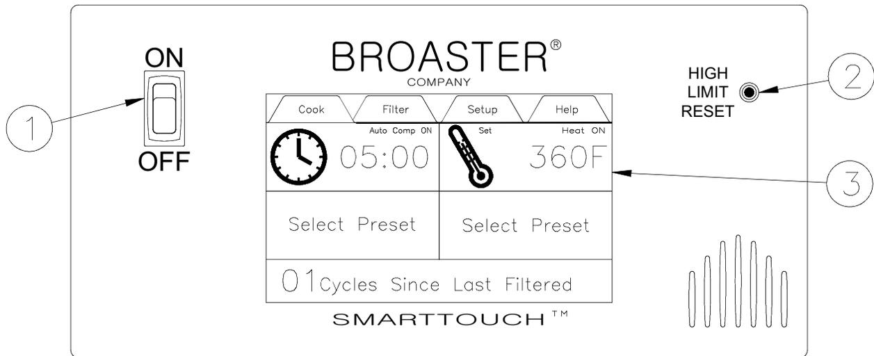
1. **Power Switch:** This switch has two positions: ON or OFF.
