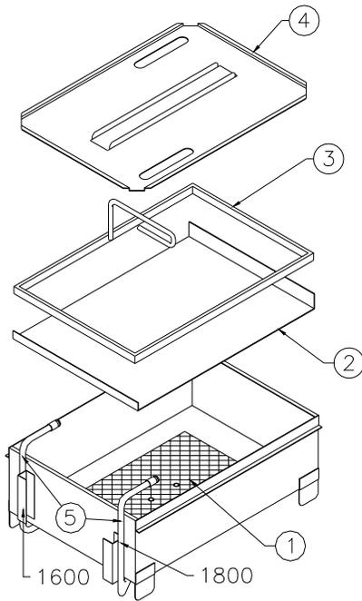
Be sure filter components are assembled correctly. Correct order is (1) Filter Screen on bottom of filter pan, (2) Filter Paper, (3) Filter Hold Down, one cup (1600) or two cups (1800) of Bro-Clean filter media on top of filter paper and/or 5 oz. (1600) or 10 oz. (1800) of XL filtering compound to cooking well, and (4) Filter Cover. For best results change paper after each filter cycle.
