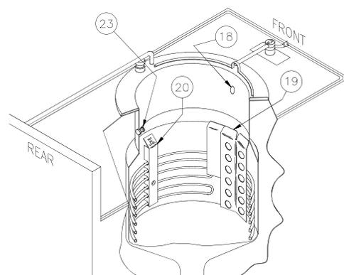
18. **Pressure Port:** When cover is CLOSED while cooking, all steam passes through this port into the pressure regulating valve.
