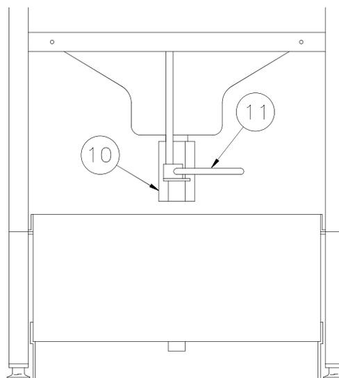
10. **Drain Valve:** Used to drain cooking oil from cooking well into filter pan or container made for handling hot oil.
