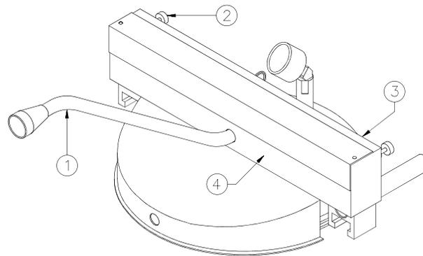
4. Slide splash shield (4) forward and up towards the end of the cover handle (1).
