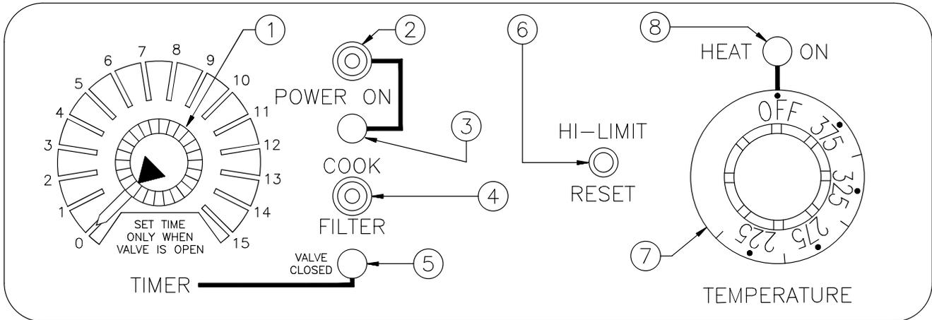
1. **Timer:** Outer dial indicates desired cooking time. Inner pointer indicates time countdown during a cook cycle.
