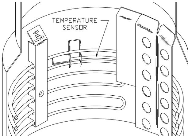
Slowly agitate brush in oil to dislodge any crumbs caught in it. Rinse cooking well using oil remaining in brush when dipped in oil. Drain remaining oil and crumbs. Pull cover over cooking well but **DO NOT CLOSE**. Turn cook/filter switch to **FILTER**. After 5 minutes, push cover assembly toward the rear of the unit. Close drain valve.
