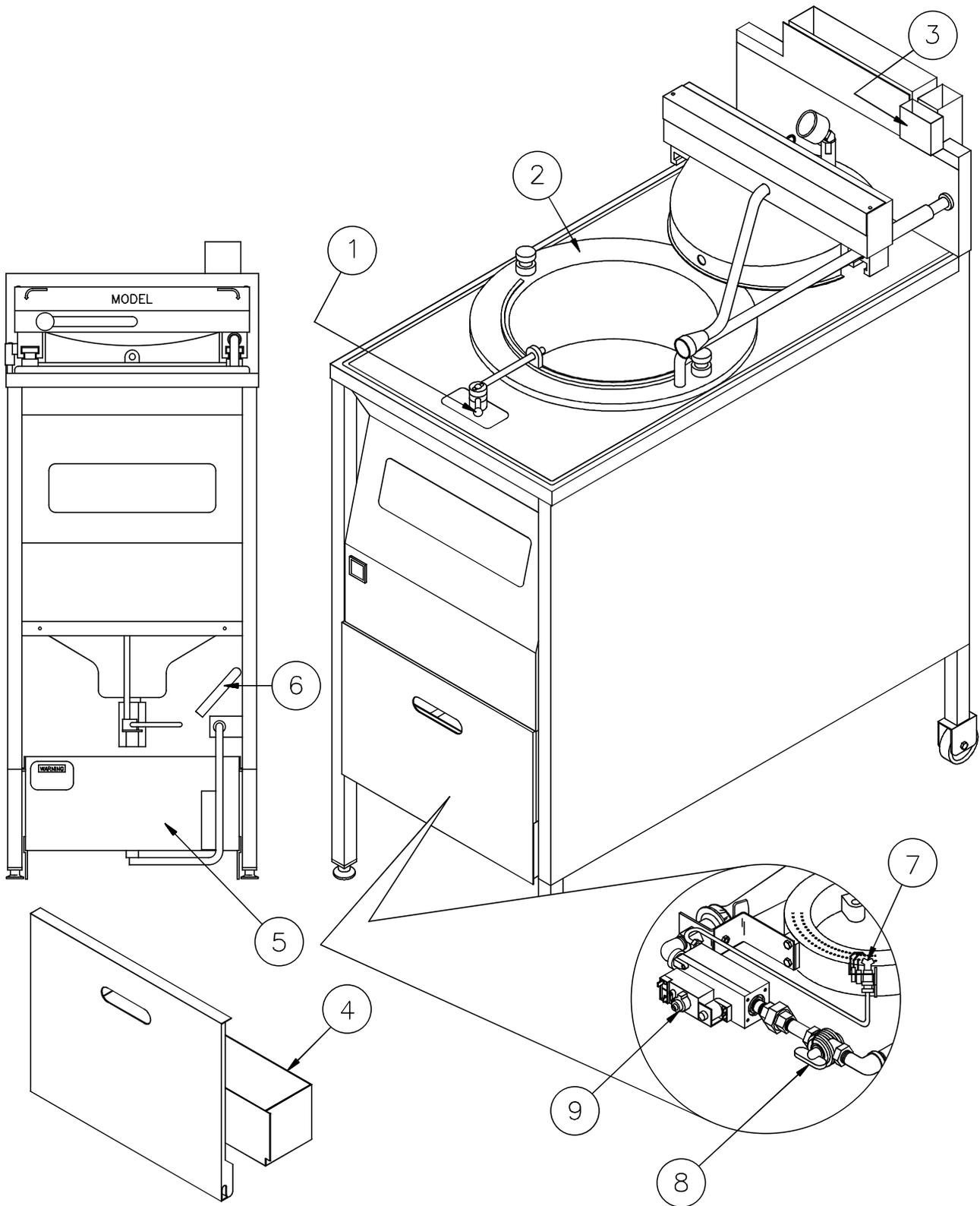
1. **Pressure Regulating Valve:** Opens and closes pressure regulating valve. When cover and valve are CLOSED, this valve seals the cooking well allowing pressure to build up. Valve is pre-set to maintain pressure at 12-14 PSI during a cooking cycle. When OPEN, all pressure is exhausted and timer stops timing.
