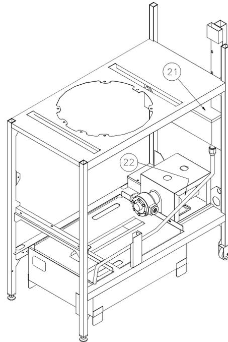
21. **Exhaust Tank:** Steam and vapors are exhausted through this tank.
