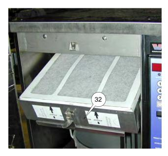
Unlatch filter cartridge (32) and pull out as shown. Check across terminals.
