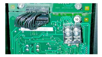
Disconnect Hi-Limit Probe wires (R & Y) form Hi-limit switch (11).
