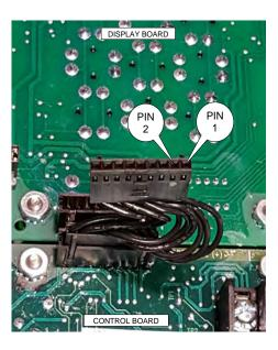
To determine if there is power to the upper Display Board, pull the plug out of the socket on the Display Board as shown above.
