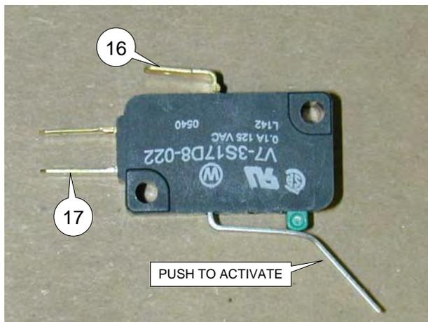
4. With the switch in its actuated position check across terminals (16) and (17) with an ohmmeter. Meter should indicate a closed circuit. If not, switch is faulty.
