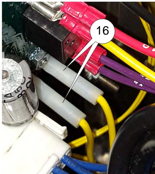
Turn the unit on and check the output voltage from these leads. It should be 24 VAC.
