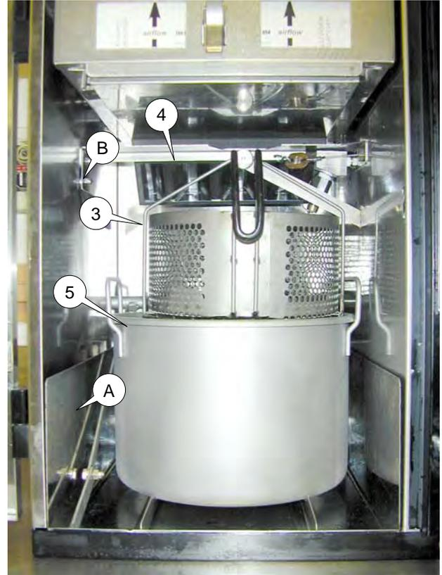
5. Raise the element by raising the element arm (A) and placing it above element retainer (B).
