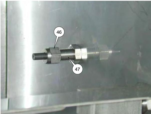
5. Pull switch and leads out of mounting fitting (47).
