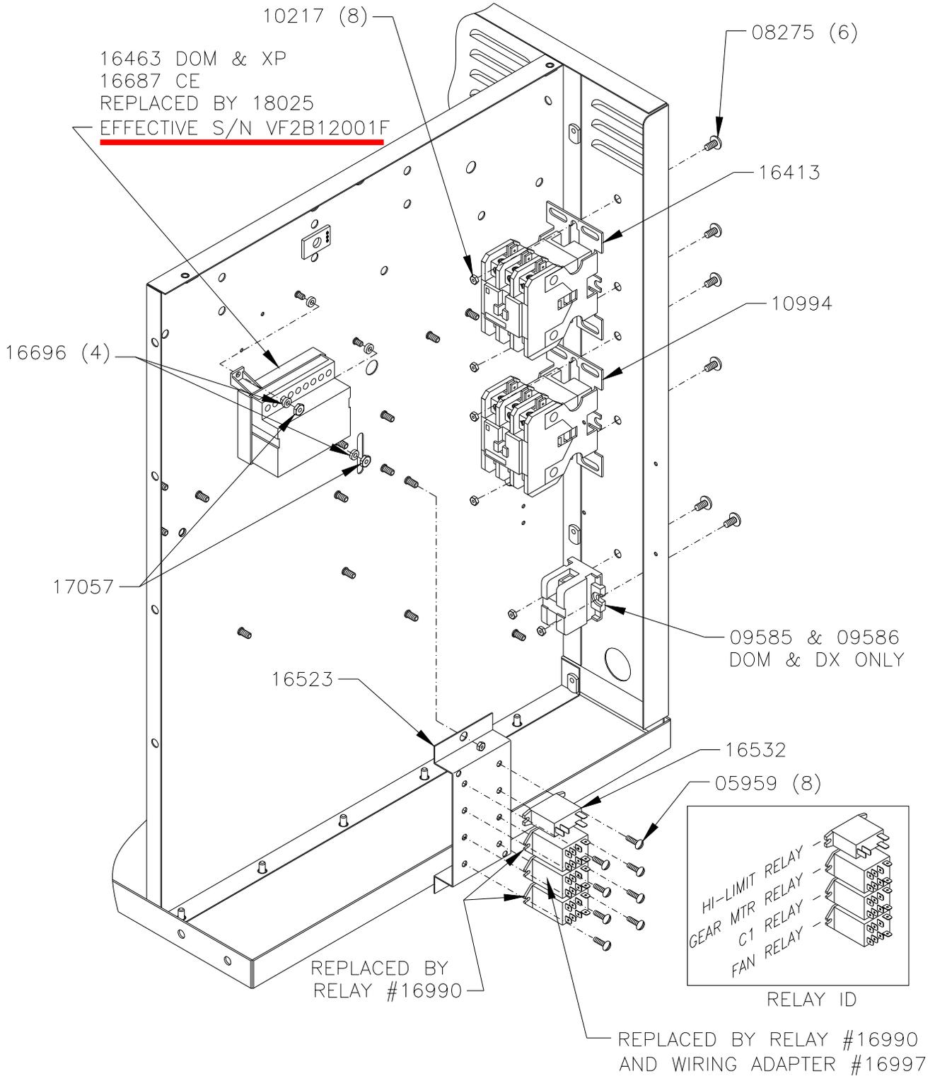
**CONTACTOR AND RELAY MOUNTING - VF2: (effective S/N VF2L900172)**
