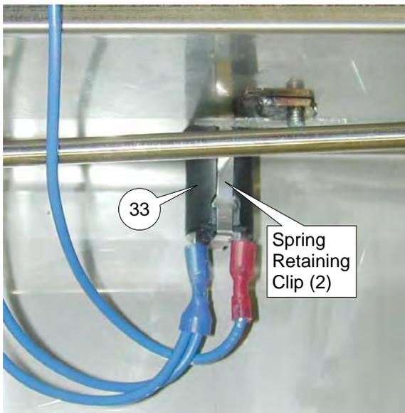
3. Disconnect wires from Air Filter Switch (33).
