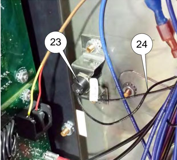
3. With product door propped open, check across wire leads (24). Meter should indicate an open circuit. If not switch is faulty.
