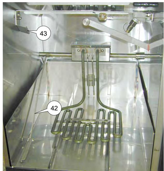
4. Raise Element Arm (42) and set it in Element Retainer (43). Check across wire leads (40). Meter should indicate an open circuit. If not, switch is faulty.
