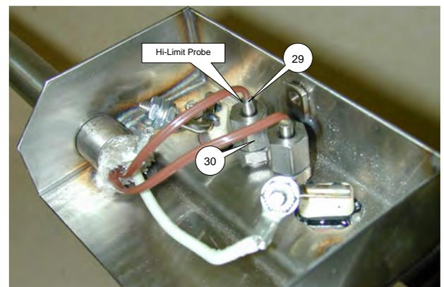
6. Install new probe in the same location as old probe. End of probe sheath should be 1/8" above nut (30) when installed properly.
