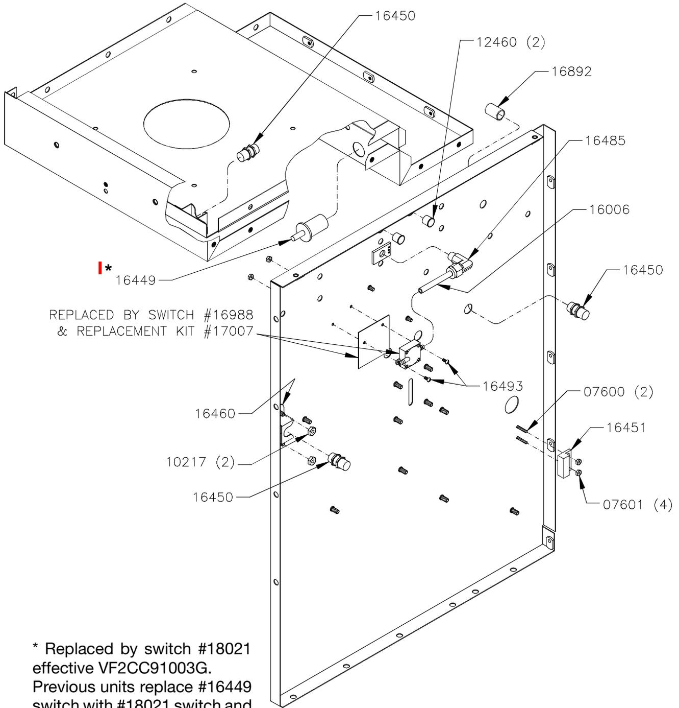
\* Replaced by switch #18021 effective VF2CC91003G. Previous units replace #16449 switch with #18021 switch and #18022 mounting plate.
