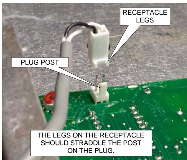
**CAUTION** The plastic receptacle (13) on the speaker wire and the plastic terminal on the control board are polarized. Make sure the receptacle on the speaker wire is attached to the control board as shown above to eliminate any problems with operation of the unit.
