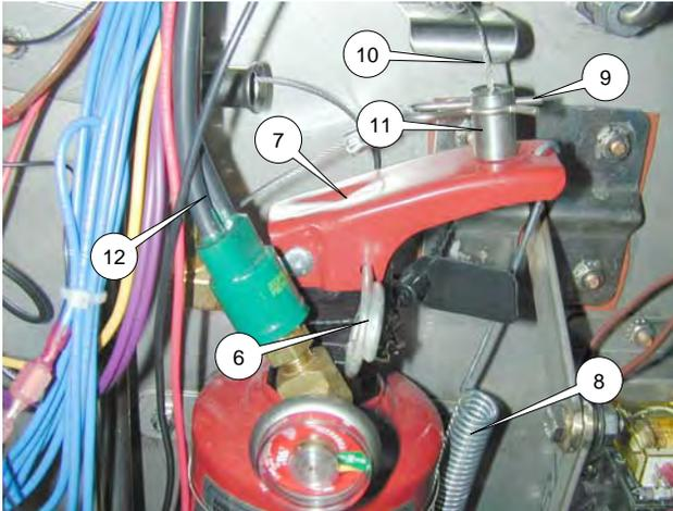
3. Release the extension spring (8) from the actuating lever (7).
