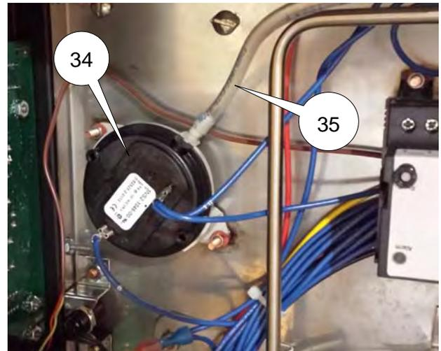
Pressure Switch (34) is mounted on two studs on the interior wall and held in place by two nuts.
