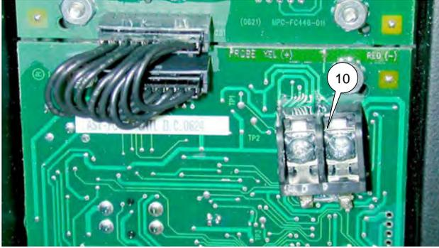
8. Disconnect Hi-Limit Probe wires (R & Y) from Hi-limit switch (11).
