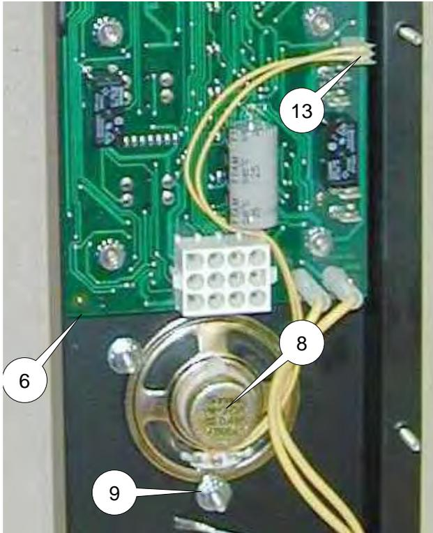
3. Check across the terminals in speaker wire receptacle with an ohmmeter. Meter should indicate a closed circuit. If not, speaker is faulty.
