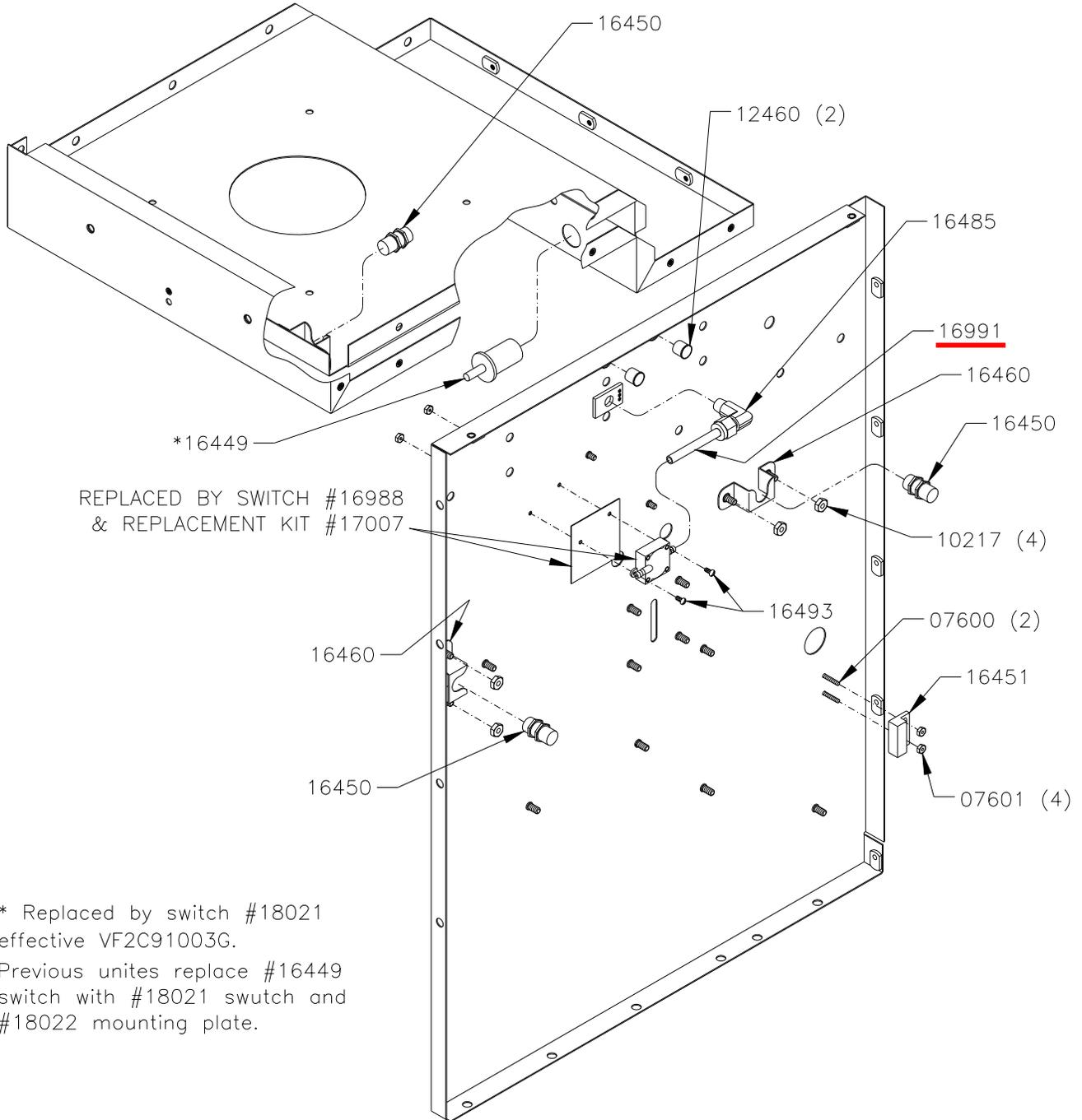
\* Replaced by switch #18021 effective VF2C91003G. Previous units replace #16449 switch with #18021 switch and #18022 mounting plate.
