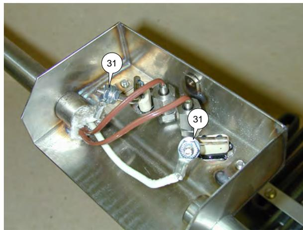
3. Remove screws (32) and remove Heating Element from Connector box (18).
