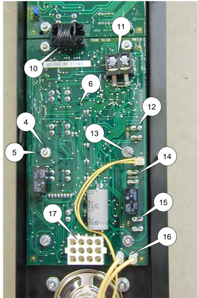
2. Disconnect jumper cable (10) at upper edge of control board.
