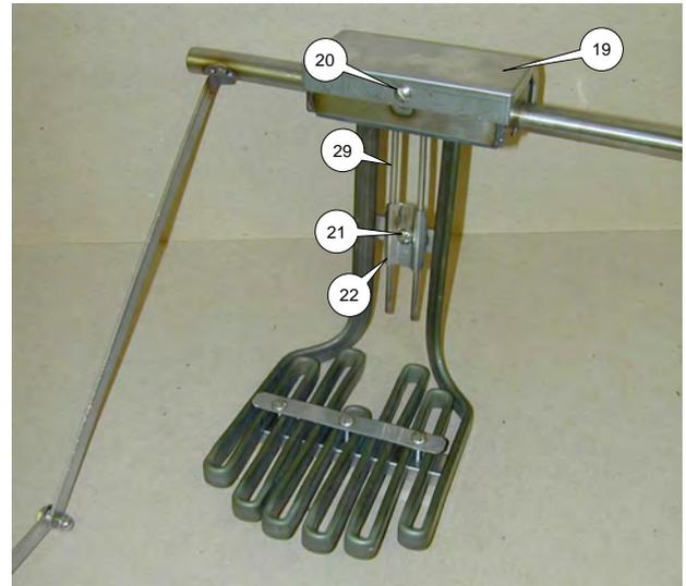
3. Remove screw (21) from probe retainer (22).
