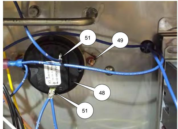
3. Remove hex nuts (49) and carefully remove tubing (50).
