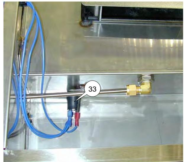
2. Disconnect wires from switch (33). Check across terminals. Meter should indicate an open circuit. If not, switch is faulty.
