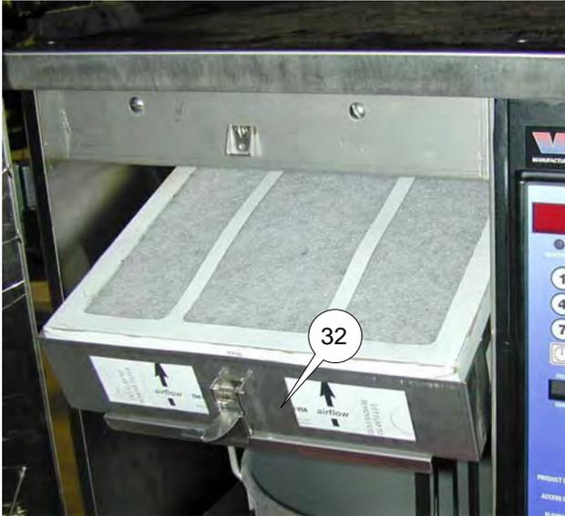
3. Unlatch filter cartridge (32) and pull out as shown. Check across terminals. Meter should indicate a closed circuit. If not, switch is faulty.
