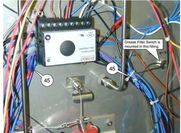
3. Unlatch Filter Tray (32) and remove from cooking compartment. Check across wire leads (45). Meter should indicate an open circuit. If not, switch is faulty.
