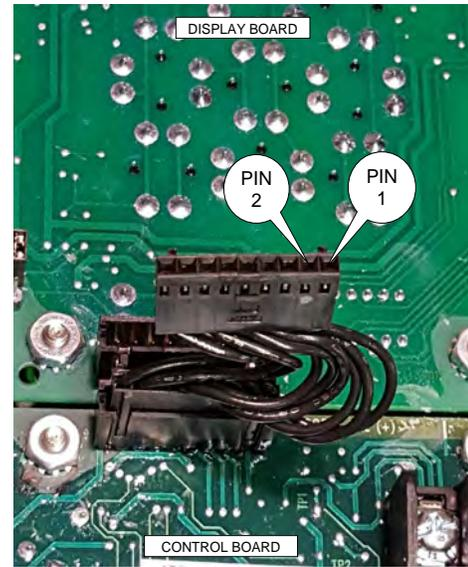
To determine if there is power to the upper Display Board, pull the plug out of the socket on the Display Board as shown above.
