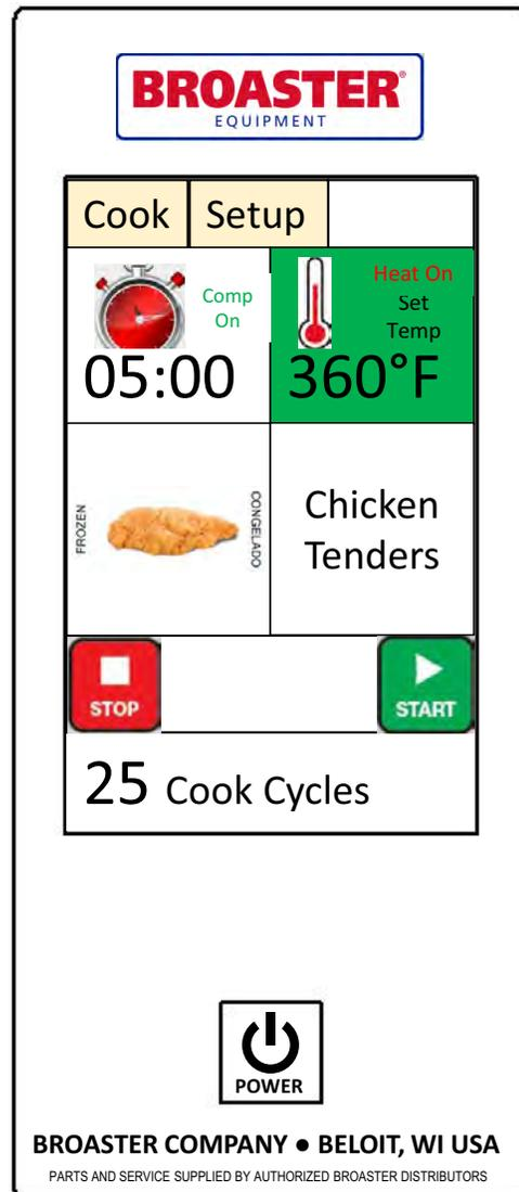
The cooking idle screen displays the current settings for time and temperature along with the recipe item that is selected. The temperature display background will turn from yellow to green when the fryer reaches the set point temperature. The display also indicates when the heat is on.
