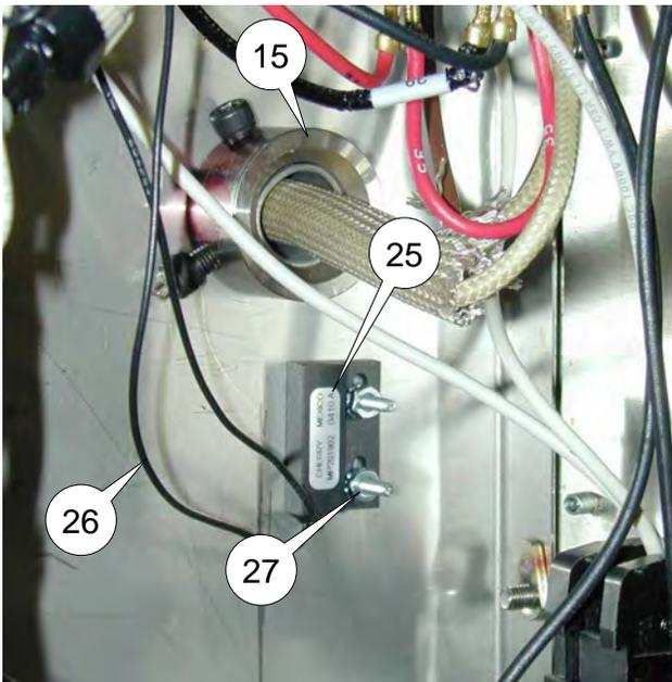
The Element Up Switch (25) is located in the control compartment on the interior wall below the element pivot shaft (15).
