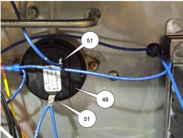
3. Remove hex nuts (49) and hose (50) from switch and remove switch from unit and clip meter leads to switch terminals (51).
