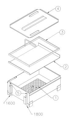
Be sure filter components are assembled correctly. Correct order is (1) Filter Screen on bottom of filter pan, (2) Filter Paper, (3) Filter Hold Down, one cup (1600) or two cups (1800) of Bro-Clean filtering media on top of filter paper and/or 5 oz. (1600) or 10 oz. (1800) of XL filtering compound to cooking well, and (4) Filter Cover. For best results change paper after each filter cycle.
