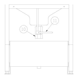
10. **Drain Valve:** Used to drain cooking oil from cooking well into filter pan or container made for handling hot oil.
