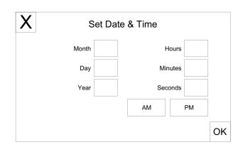
To set the date and time, press the box after "Month" and a keypad will appear. Enter the number of the month and press the enter key. Repeat this action for the Day, Year, Hours, Minutes, Seconds, AM and PM boxes. When finished press the green OK button. To leave this display without making a change press the red X or the green OK.
