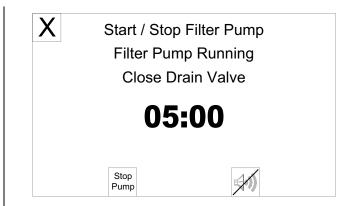
Press STOP PUMP after the oil is completely returned to the cooking well or you can leave the pump running and it will automatically stop when the counter says 10:00 minutes. See display below.
