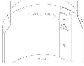
**ACAUTION** Using too much force in this area could result in damage to either the hi-limit capillary or the temperature sensor probe. If either of these components are damaged, the unit will be inoperable until the component is replaced.
