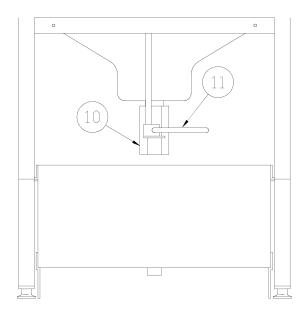
10. **Drain Valve:** Used to drain cooking oil from cooking well into filter pan or container made for handling hot oil.
