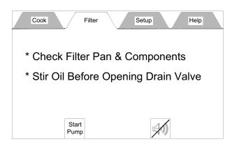
This tab is the filter motor control and has two buttons; a Start Pump button and a Silence Alert button.
