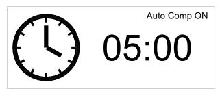
The cook time is indicated in the box next to the clock face. To change the time press the time display twice and a keypad will appear.
