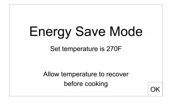
When the OK button is pressed the display returns to the normal Cook Tab display and the temperature will be yellow and Low and the set temp will be alternating. **DO NOT** start cooking until the temp display is green.
