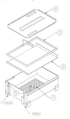
Be sure filter components are assembled correctly. Correct order is (1) Filter Screen on bottom of filter pan, (2) Filter Paper, (3) Filter Hold Down, one cup (1600) or two cups (1800) of Bro-Clean filtering media on top of filter paper and/or 5 oz. (1600) or 10 oz. (1800) of XL filtering compound to cooking well, and (4) Filter Cover. For best results change paper after each filter cycle.
