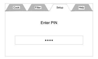
3. Press the box with the four stars in the middle and when the keypad appears enter service PIN code 0540 and press Enter.
