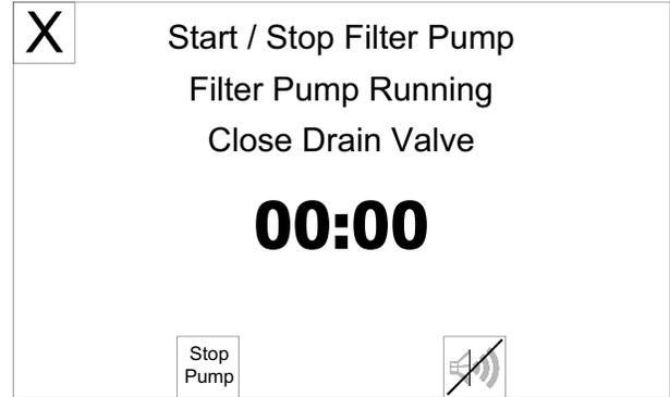
The pump will continue to run and will automatically stop when the counter says 10:00 minutes. You will see the display below.
