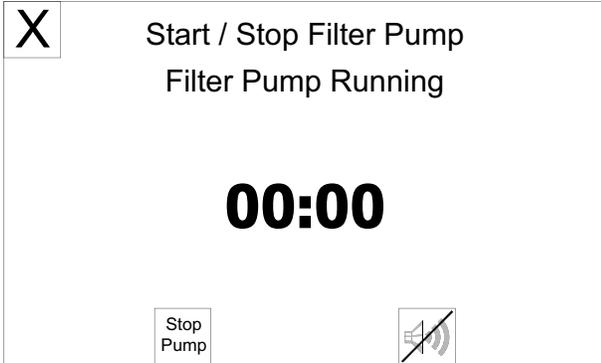
The timer in the middle of the screen starts counting up. When it reaches 5:00 minutes an alert sounds and a reminder flashes (see below) to close the drain valve. To silence the alert press the button with the speaker on it. DO NOT press the Stop Pump button.
