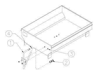
1. From bag of hardware, install compression nut then 2 piece ferrule onto riser line (1). (see below)
