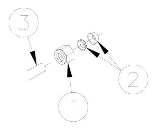
Install riser line onto pan. First install line into fitting (2) on bottom center of pan while the mounting plate fits over studs (3) on front of pan.
