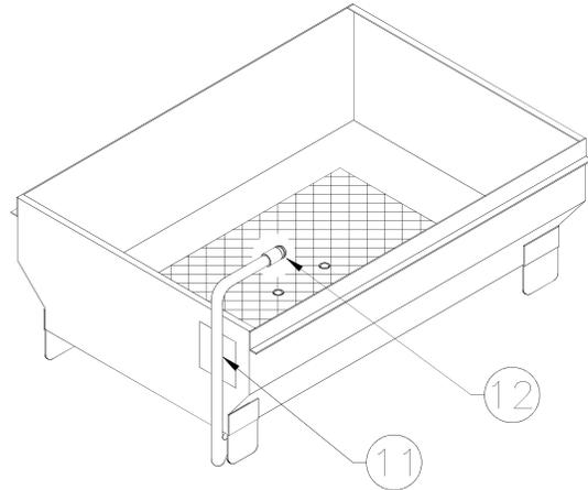
1. Use a clean cloth or paper towel to wipe crumbs from filter hold down and the filter pan interior before replacing filter paper. This will help prevent crumbs from causing a poor seal or entering the riser line (11) and pump.
