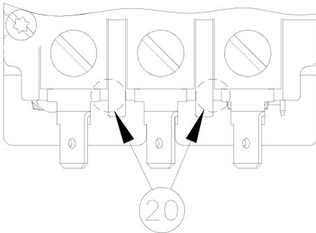
9. If any contactor will not close electrically, check coil (20) with an ohmmeter. With needle nose pliers, disconnect wire(s) from one side of the coil. Meter should indicate a closed circuit. If not, coil is faulty.
