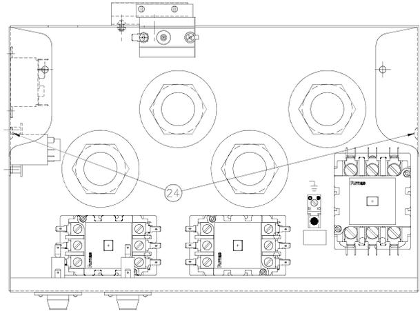
9. Pull Power Input Box forward. You may have to remove the locknut from the conduit fitting on the left side of the box, as well as any wires that prevent you from moving the box far enough to access the element mounting nuts.
