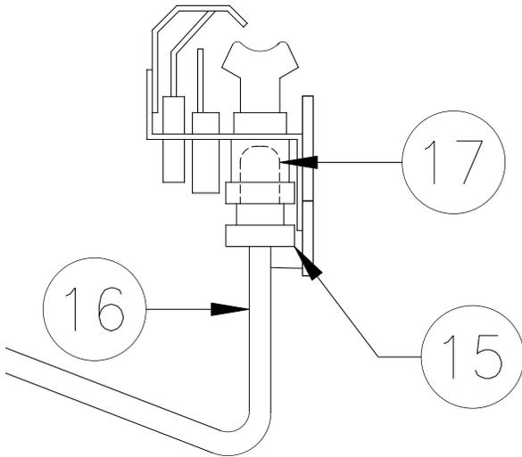
Orifice (17) is located above brass fitting (15).
