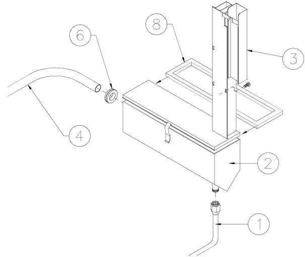
1. Remove exhaust drain tube (1) from bottom of the tank (2).
