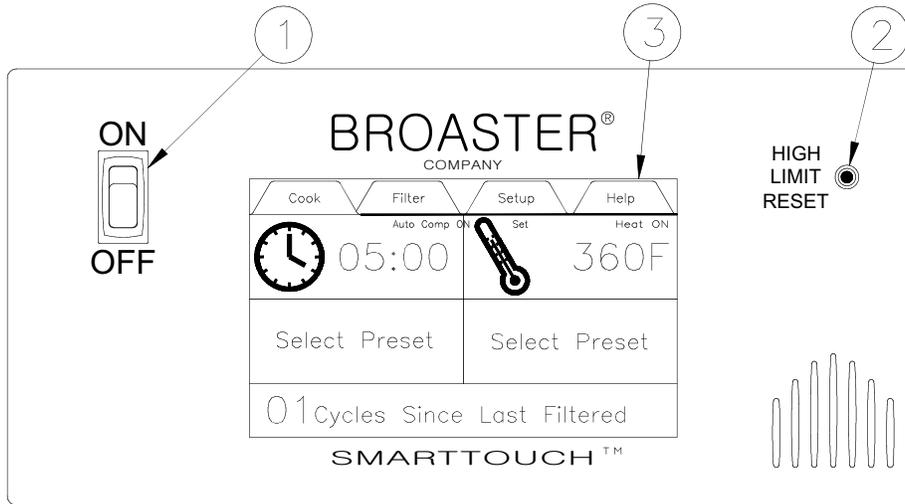
**1. Power Switch:** This switch has two positions: ON or OFF.
