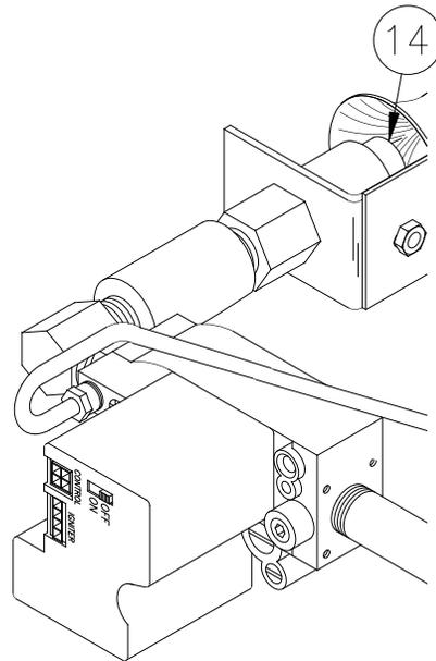
9. Assemble in reverse order. Check all connections and pipes with a soap and water solution. Bubbles indicate a gas leak.
