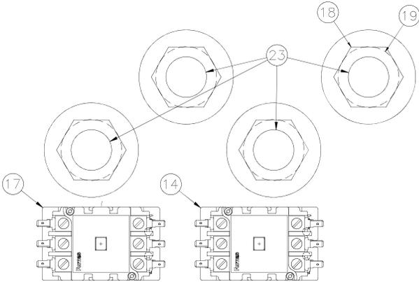
2. Disconnect all suspected element wires from contactor.
