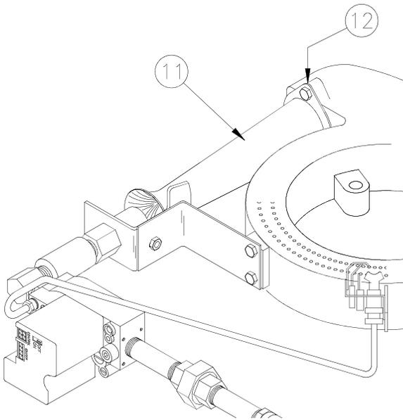
5. Loose venturi (11) or bad gasket (12) can affect combustion. Tighten or replace gasket.
