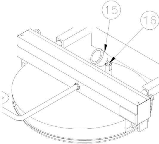
2. Unscrew gauge (15) from the elbow (16).
