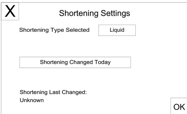
Pressing the button next to Shorting Type toggles between “Liquid” and “Solid”.
