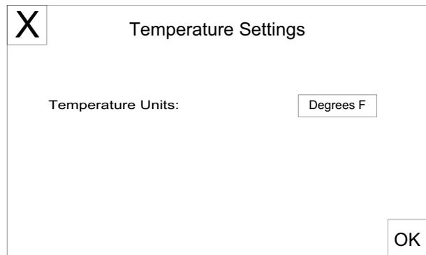
Pressing the Degrees box switches the units. Then press OK.
