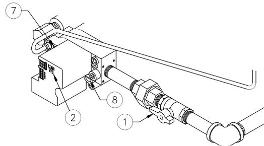
1. Turn power switch, manual gas shut off valve (1) and switch (2) OFF.
