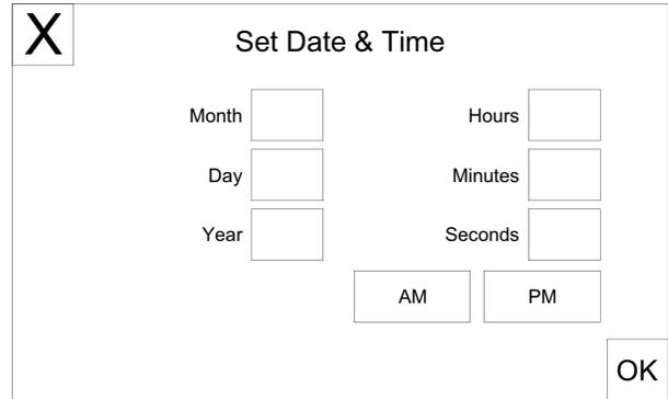
To set the date and time, press the box after "Month" and a keypad will appear. Enter the number of the month and press the enter key. Repeat this action for the Day, Year, Hours, Minutes, Seconds, AM and PM boxes. When finished press the green OK button. To leave this display without making a change press the red X or the green OK.
