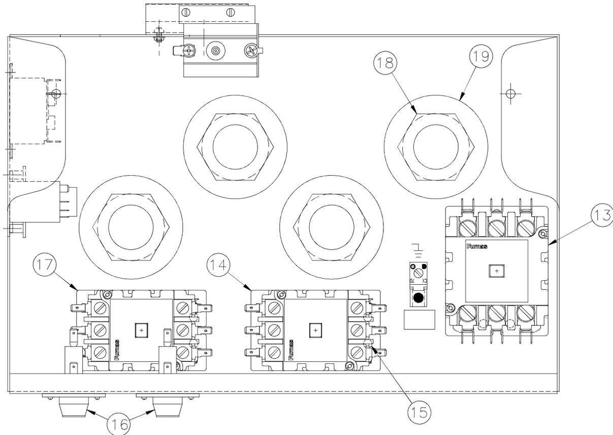
The 2400E has a pre-heat circuit that controls Secondary Contactor (17). When the 2400E is turned on for the first time the pre-heat circuit keeps the upper element from energizing until the oil temperature reaches set point. If more than ten seconds elapses before the next call for heat the upper elements will energize when the HEAT ON indicator in the Temperature section appears.
