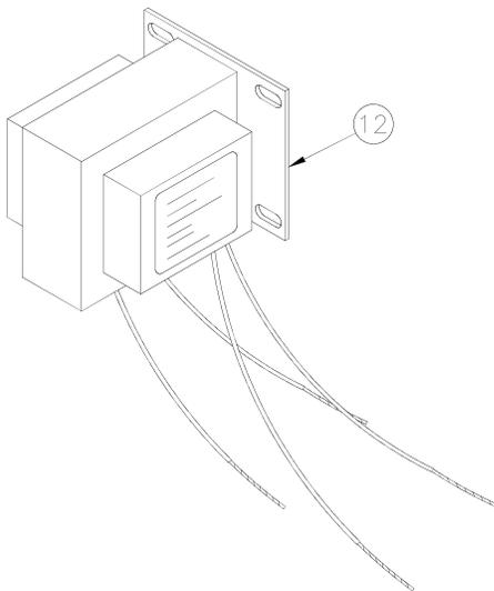
2. Disconnect one wire from the primary (black and white wires) side and secondary (yellow and blue wires) side of the transformer.
