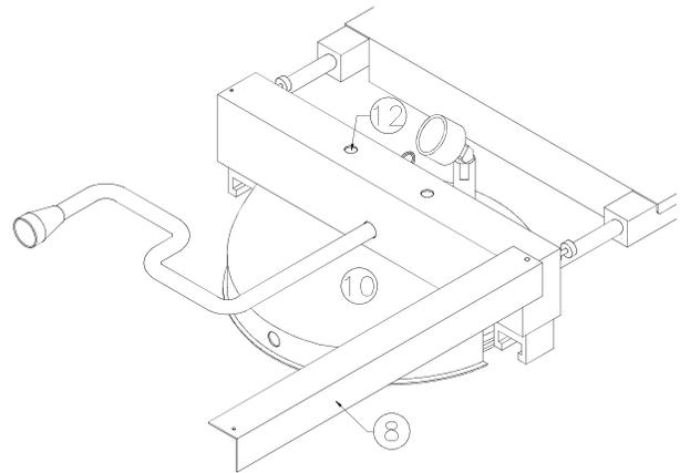
1. Remove screw from left side of warning sign (8) and swing out toward the right.
