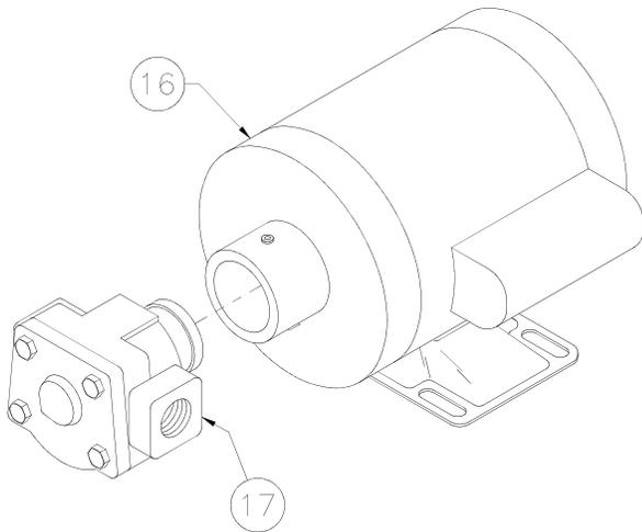
Motor (16) turns pump (17) which returns cooking oil from filter pan to the cooking well.
