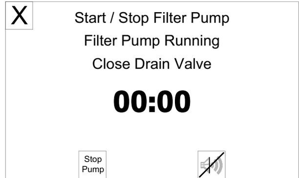
Press STOP PUMP after the oil is completely returned to the cooking well or you can leave the pump running and it will automatically stop when the counter says 10:00 minutes. See display below.
