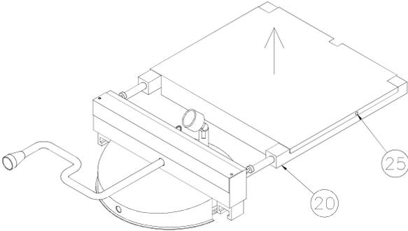
2. Remove two thumbscrews (25) attaching the lift assembly cover and remove from assembly (20). Remove cover drip pan.
