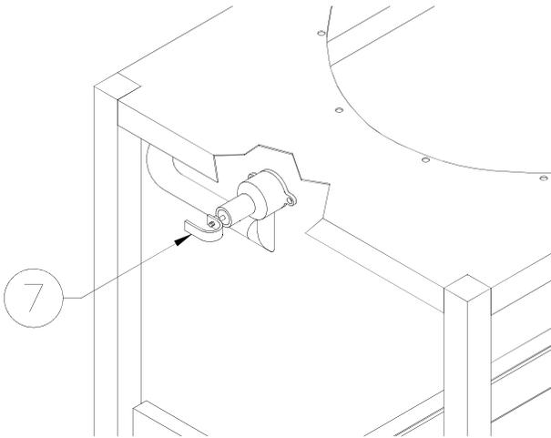
Valve (7) is preset to maintain a maximum pressure of 12-14 psi during a cooking cycle. Pressure may build slowly or remain low when cooking small loads. Add one or two quartered potatoes with product to help build and maintain maximum pressure.
