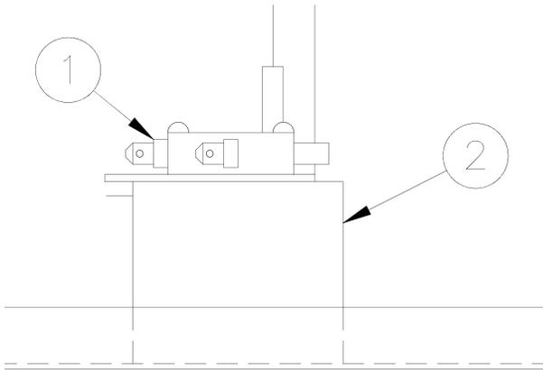
2. With needle nose pliers, disconnect one wire from the switch (1).
