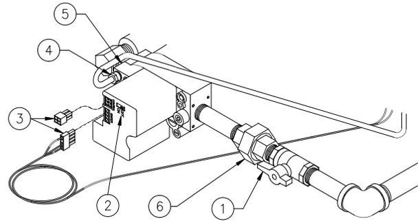
1. Turn power switch, manual gas shut off valve (1) and switch (2) OFF.
