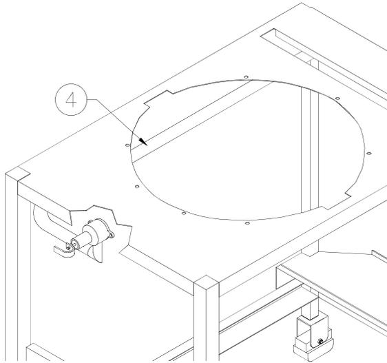
Tube (4) directs steam and vapors from cooking well into the exhaust tank.
