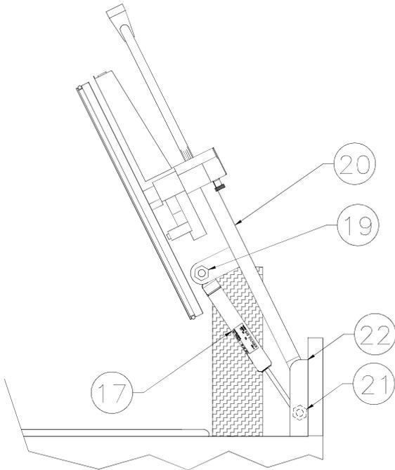
3. Raise the cover to its full open position and place a solid support under the lift to keep it in raised position.
