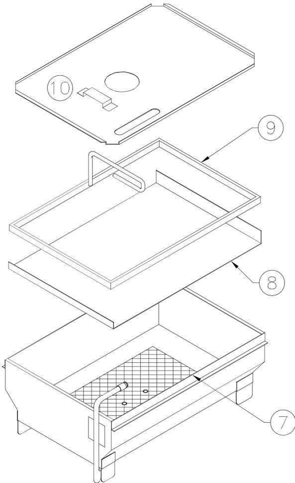
Be sure filter components are assembled correctly. Correct order is filter screen (7) on bottom of filter pan, filter paper (8), filter hold-down (9), 3 cups of Broaster® filtering compound on top of filter paper and cover (10) on filter pan.
