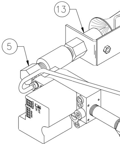
6. Loosen union elbow (5) and remove locknut (13).
