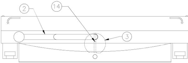
2. Install handle (2) through splash guard, into yoke bar then into the cam.
