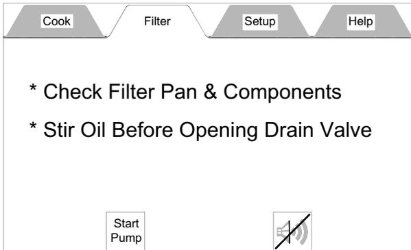
This tab is the filter motor control and has two buttons; a Start Pump button and an Alert Silence button.
