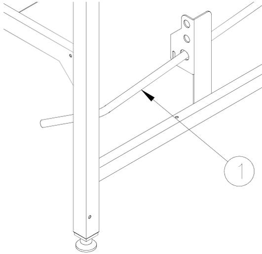
Tube (1) drains condensation from exhaust tank into the condensate pan.
