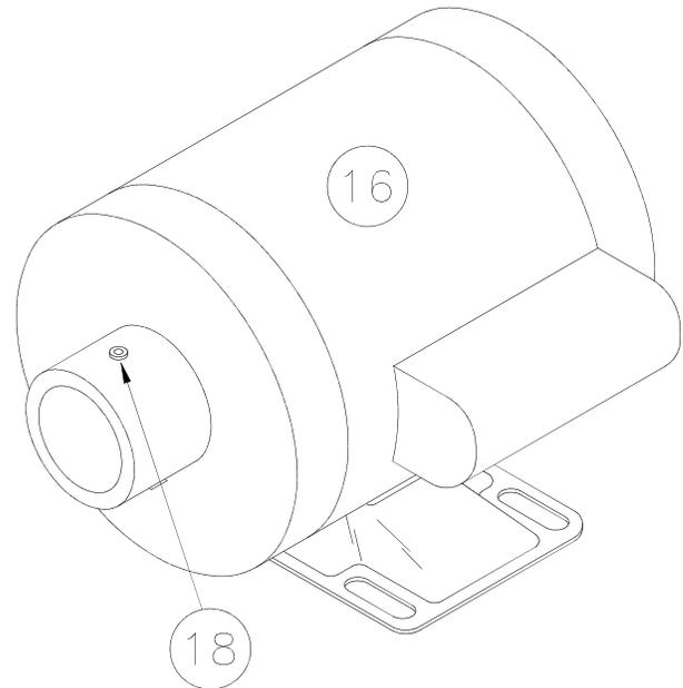
3. Loosen three set screws (18) in neck of motor (16) which hold pump in place.
