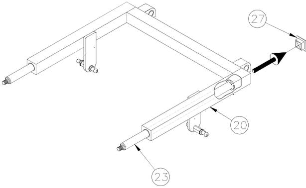
2. Remove the slide rod (23) from the lift assembly (20) by sliding in the direction of the arrow.
