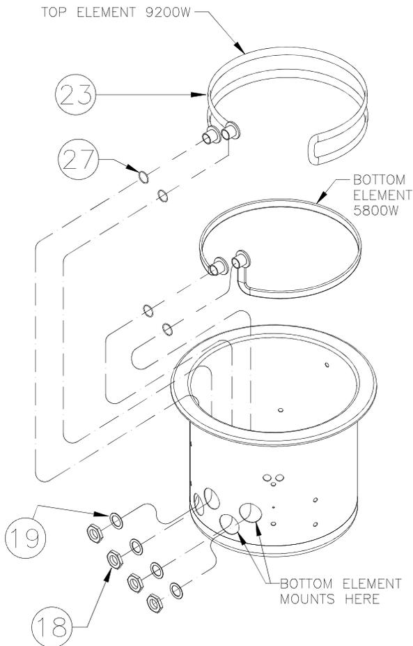
15. Install new elements using new gaskets (27) located between element and inside of the cooking well bulkhead.
