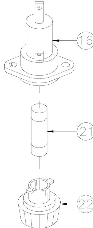
2. With needle nose pliers, disconnect wire(s) from one end of fuse holder (16).
