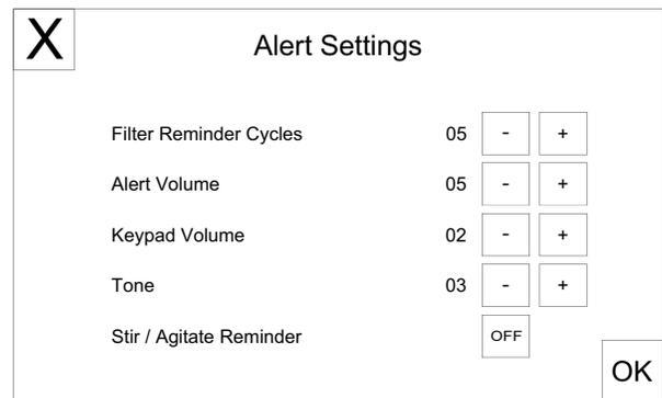
The numbers left of the boxes indicate the current setting. They can be changed by pressing the “-” or “+” buttons.
