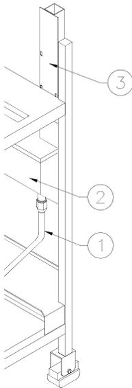
See previously mentioned operator habits. Muffler (2) can become obstructed. The obstruction usually forms on the bottom of tank where exhaust drain tube (1) is connected. Tank will then become filled with liquid. Liquid may be forced up the stack (3) when pressure is released at the end of a cooking cycle.
