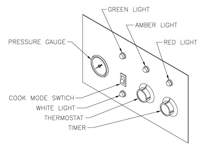
**PRESSURE GAUGE:** Indicates the pressure in the Cooking Well.
