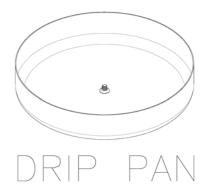
Place drip pan in bottom of cooking well. If cooking well is hot, place drip pan in cooking well by using the spit. Then remove spit by unscrewing counter-clockwise leaving the drip pan in bottom of cooking well.
