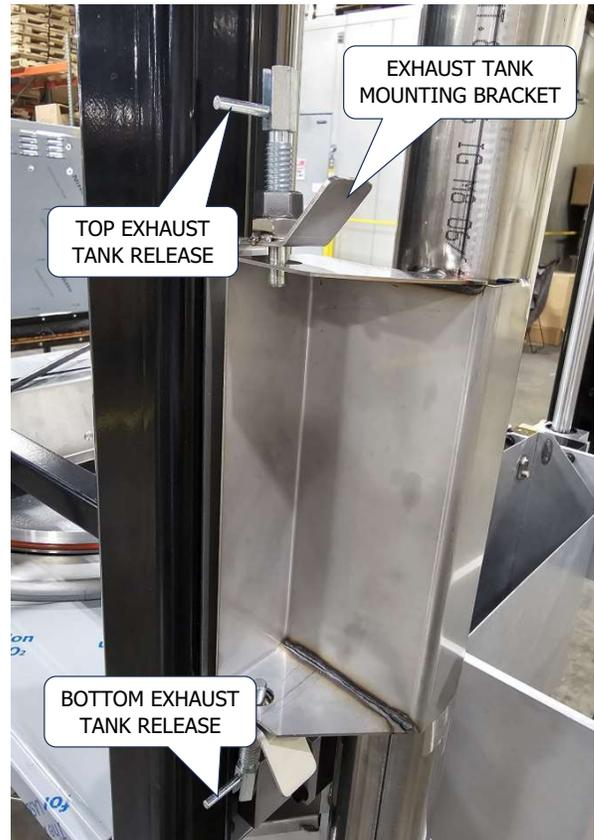
3. Pull the stack out of the mounting bracket. Then pull the exhaust tank off of the exhaust tube.
