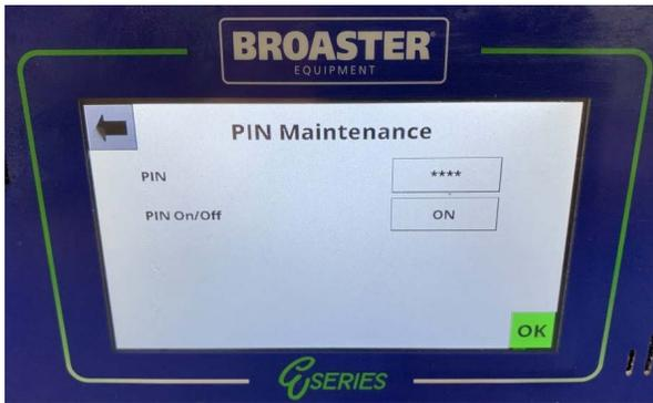
When the unit is installed there is no PIN set. To set a pin press the box next to PIN and the key pad screen will appear. Set the 4 digit pin you want and press enter. Press the box next to PIN on/off to turn the PIN on.
