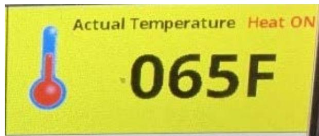
When the fryer is turned on in the morning this box will be yellow and “Heat On” will be displayed. The temperature will alternate between “LOW” and the set temperature until the oil temperature reaches the set temperature.
