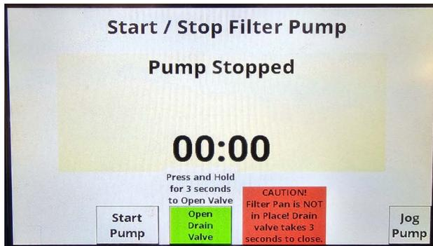
If the filter pan is in place, the Filter in Place, Okay to proceed field will be highlighted.
