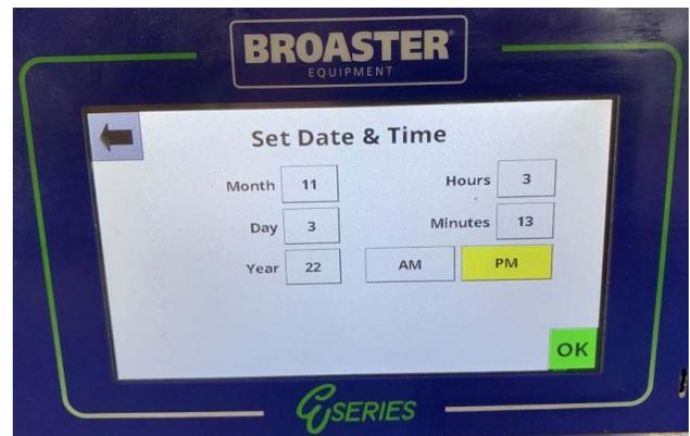
To set the date and time, press the box after "Month" and a keypad will appear. Enter the number of the month and press the enter key. Repeat this action for the Day, Year, Hours, Minutes, AM and PM boxes. When finished press the green OK button or the changes will not be saved.
