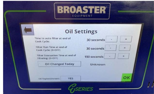
The recirculation time for the auto-filter feature can be adjusted here in 10 second intervals. The filter evacuation time at the end of auto-filtering can also be adjusted in 30 second intervals.
