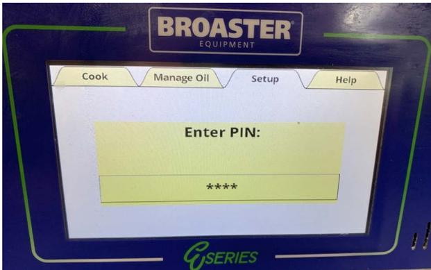
If the Pin number is known, press the box and a keypad will appear. Enter the PIN number and press Enter.
