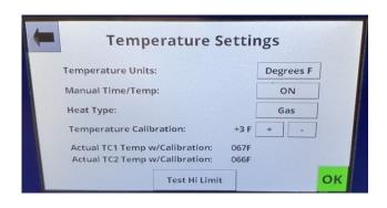
The temperature scale can be set in this display to either Degrees F (Fahrenheit) or Degrees C (Celsius).
