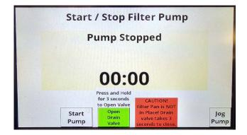
If the filter pan is in place, the Filter in Place, Okay to proceed field will be highlighted.
