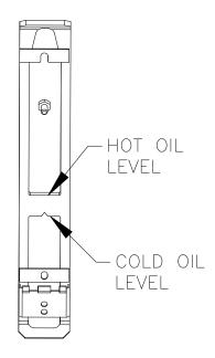
Hot Oil Level: Indicates proper level when oil is at operating temperature. HOT OIL level is indicated by top line and cold oil fill is indicated by lower line on all 3 inner well guards.
