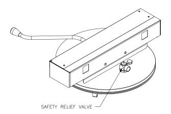
15. Safety Relief Valve: This valve will open in the event pressure in the cooking well meets the relief pressure of valve. A properly installed valve has the outlet facing toward rear corner of the countertop. **DO NOT** use valve to release pressure at the end of a cooking cycle. If valve leaks during normal operation, **DO NOT** operate the unit until valve is replaced by an authorized Broaster Company representative.
