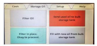
When the red field is touched, the drain and rear disposal valves will open and the pump start screen will appear.
