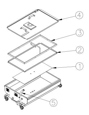
Be sure filter components are assembled correctly. Correct order is (1) Filter Screen on bottom of filter pan, (2) Filter Paper, (3) Filter Hold Down, 3 cups of Bro-Clean filtering media on top of filter paper and/or add 15 oz. of XL filtering compound to cooking well, and (4) Filter Cover. For best results change paper after each filter cycle.
