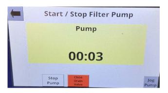
The timer in the middle of the screen starts counting up. When the timer reaches 5:00 minutes an alert sounds and a reminder flashes. To silence the alert, press the button with the speaker on it.
